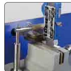
lapping measuring surfaces of caliper lower jaws
