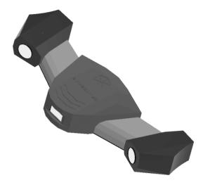
The eviXscan 3D WideRange 65 emerges as an advanced solution designed for meticulous quality control of expansive objects, tailored for dimensions ranging from 100 mm to 1200 mm. This scanner stands out for its capacity to deliver comprehensive, high-accuracy inspections swiftly, integrating seamlessly into diverse industrial frameworks.
